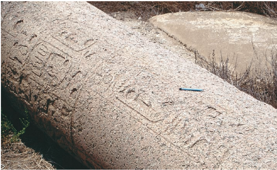
FIGURE 10.7 A column of granite from a temple in Lower Egypt fell over and its right side was partially buried for hundreds of years. Moisture in the soil facilitated hydrolysis and altered much of the feldspar to clay. The left side of the column was exposed only to the dry atmosphere and remained fresh and unaltered for more than 2000 years.
