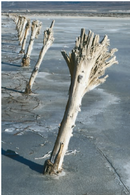
FIGURE 10.3 Growth of salt crystals has shattered these fence posts near the shore of the Great Salt Lake, Utah. Salty groundwater seeps into the wood, and, as it evaporates, salt crystals grow, expand, and break apart the wood fibers.
